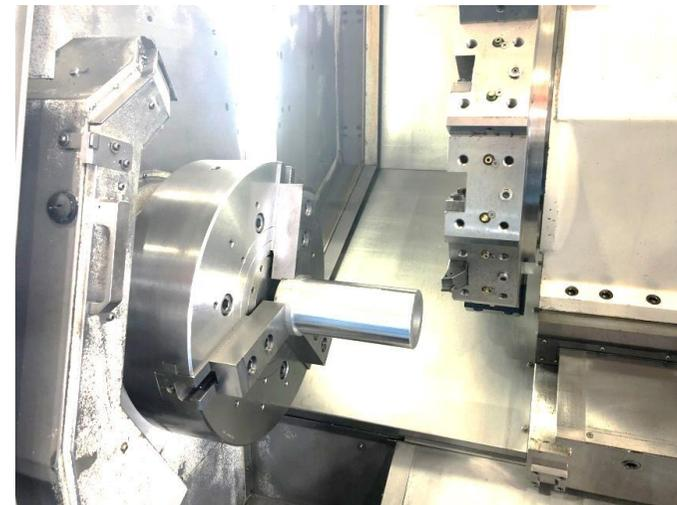
口元径104.82mm 先端径104.83mm
